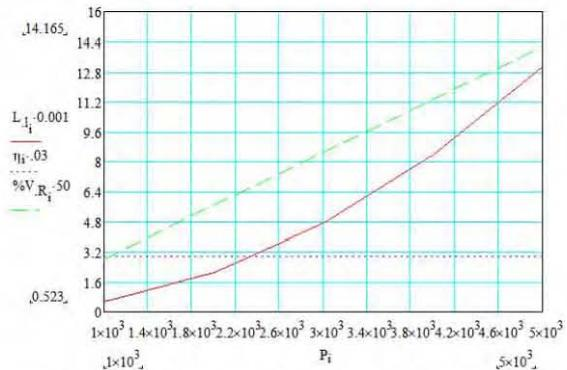
Fig.3 Result Curve for Voltage Regulation, Line Loss and Efficiency Compared with Existing and Expansion at Outgoing Feeder in Aung Pin Lae Substation
