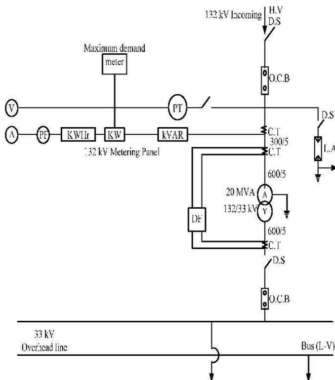
Fig. 1 Measuring System for Additional Transformer
